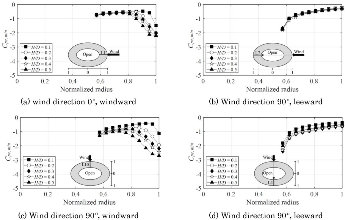
Fig. 6  $C_{pe,min}$  according to wind direction
