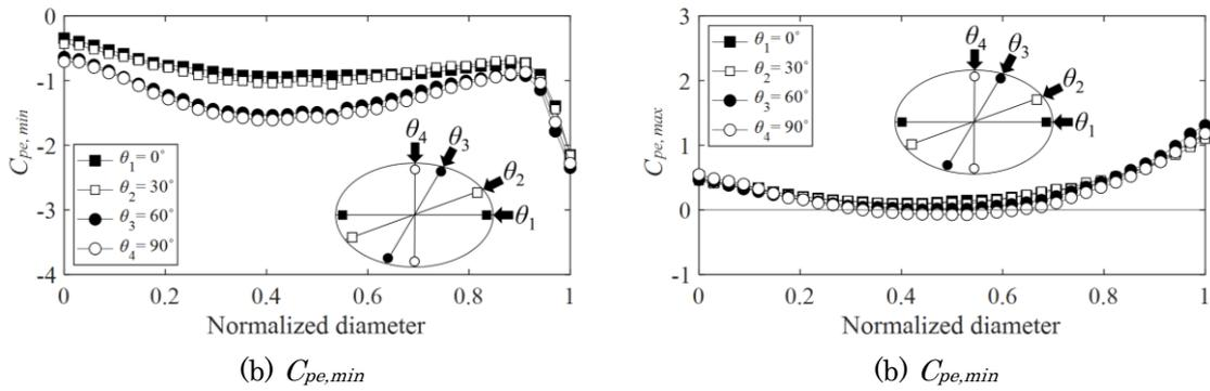
Fig. 4 Wind pressure coefficients according to wind direction
