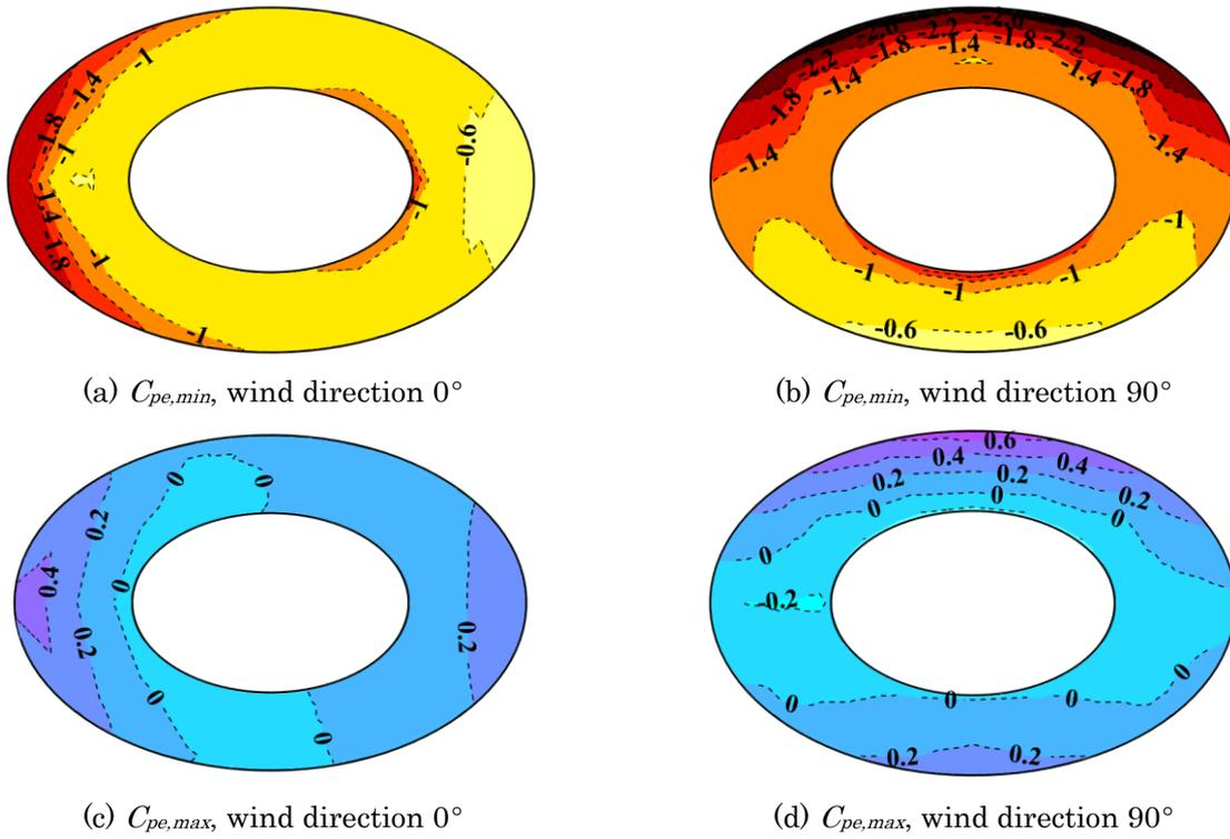
Fig. 5 distribution of  $C_{pe,min}$  according to wind direction
