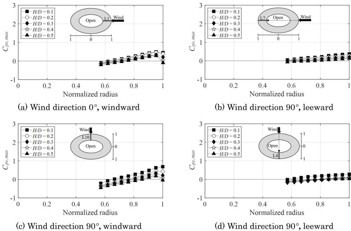
Fig. 7  $C_{pe,max}$  according to wind direction
