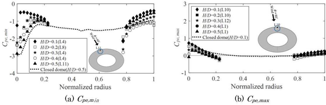
Fig. 3 Peak pressure coefficients of central open dome
